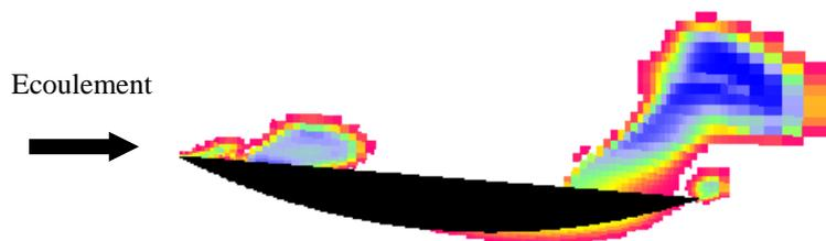
**Figure 5 :** Example of unsteady simulation of sheet cavity with a homogeneous model based on a barotropic law of state (the colours indicate the density, white for pure liquid and from red to blue when the void ratio increases)
